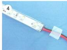
4. Put the end-cap on the end of LED strip, get the wires through the small hole.
