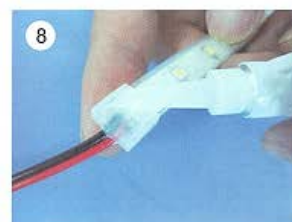
8-9. Dispense the glue on the gap between the end-cap and LED strip, and the small hole on the end-cap. Please wait for 30 minutes till the glue gets solidified.
