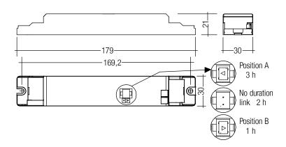
Note: Supply of control gear with duration link in 3 hours position. Duration link must be set before battery and mains connection.
