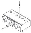
Loosen wire through twisting and pulling or using a  $\emptyset$  1 mm release tool
