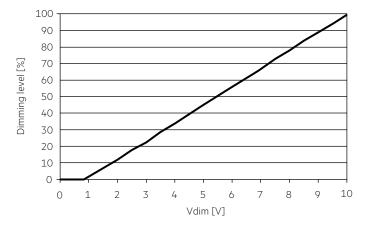
BRIDGE sends stand-by command to LMI LED Drivers from operation to stand-by for a voltage of < 0.8 V and from stand-by to on for a voltage of > 1 V.
