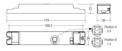
Note: LED Driver supplied with duration link in 3 hours position. Duration link must be set before battery and mains connection.
