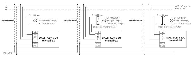
Mixed loads (capacitative, inductive and ohmic) may be used.  $^{\mbox{\tiny D}}$
