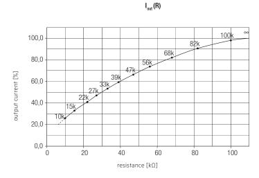
Used resistor range E12 Component tolerances are not considered in the diagram
